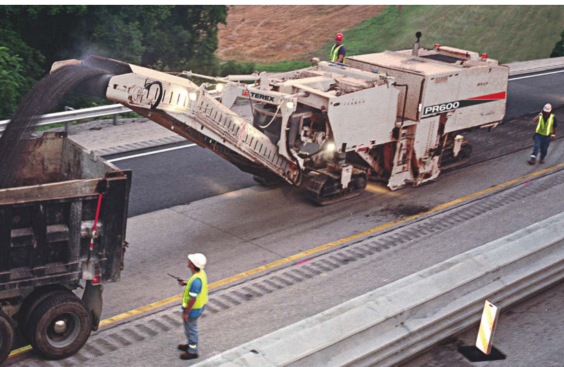
The half- and full-lane Terex Roadbuilding milling machines, including the smaller PR600C shown here, are available in either a three- or four-track configuration, with a large track in the rear for enhanced stability. Terex offers five milling model sizes, including the PR330 available in both a track and wheel configuration.
