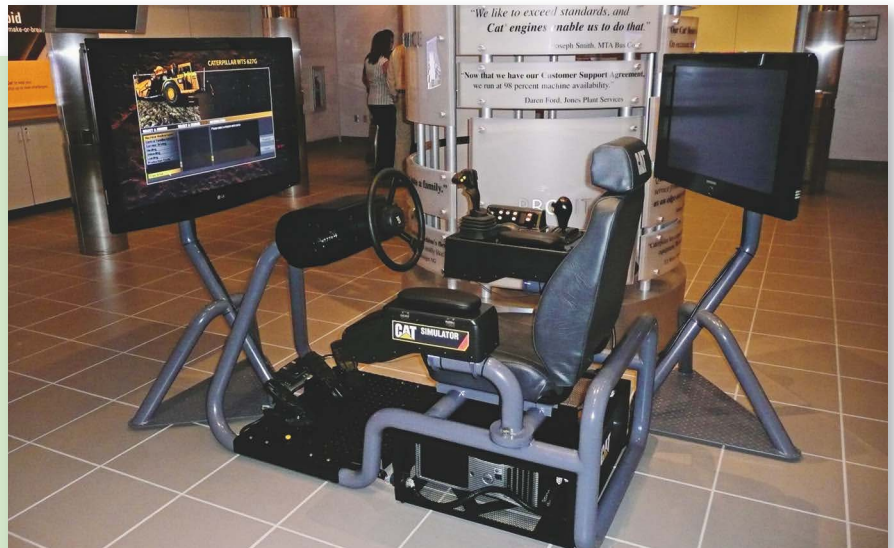
Caterpillar unveils new operator-training simulator technology. Two monitors are necessary here because of the front and rear views required while operating a wheel tractor scraper.
